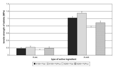
Fig. 7. Tensile strength of tablets at the compression force of 8 kN: Xylitab 100 and Xylitab 200 with active ingredients
