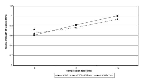
Fig. 1. Tensile strength of tablets in function of compression force: Xylitab 100 with lubricants
