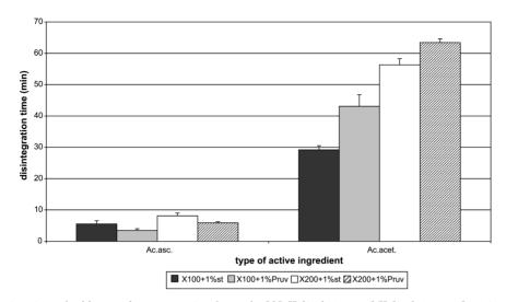
Fig. 8. Disintegration time of tablets at the compression force of 8 kN: Xylitab 100 and Xylitab 200 with active ingredients Explanations of the abbreviations used in Figures:
