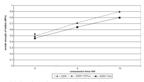
Fig. 2. Tensile strength of tablets in function of compression force: Xylitab 200 with lubricants
