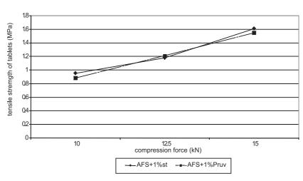
Fig. 1. Tensile strength of tablets in function of compression force: Advantose FS 95 with lubricants
