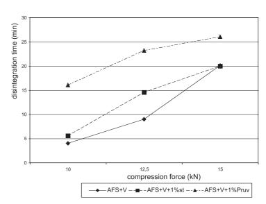
Fig. 5. Disintegration time in function of compression force: Advantose FS~95~and~Vivapur~102~in~the~ratio~of~1:1~without~and~with~lubricants
