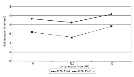
Fig. 4. Disintegration time in function of compression force: Advantose FS 95 with lubricants
