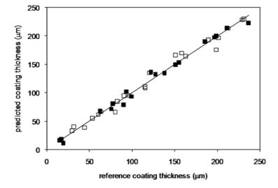
Fig. 2. The correlation plot of the reference film coating thickness (determined by microscopic analysis) and the PLS algorithm predicted film coating thickness by cross validation ( $\blacksquare$  EL,  $\square$  – ES)
