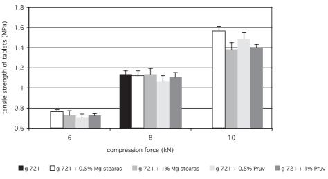
Fig. 2. Tensile strength of tablets in function of compression force: galen IQ 721 g 721 – galenIQ 721, Mg stearas – magnesii stearas
