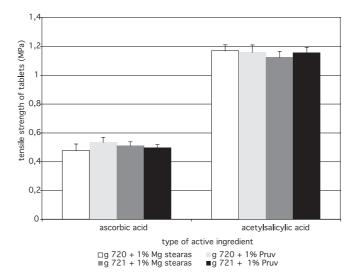
Fig. 5. Tensile strength of tablets at the compression force of 10kN: galen IQ 720 and 721 with active ingredients g 721 – galenIQ 721, Mg stearas – magnesii stearas
