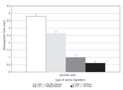
Fig. 6. Disintegration time of tablets at the compression force of 10 kN: galen IQ 720 and 721 with ascorbic acid g 720 – galen IQ 720, g 721 – galen IQ 721, Mg stears – magnesii stears
