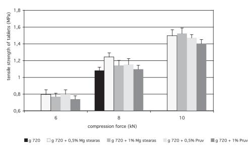
Fig. 1. Tensile strength of tablets in function of compression force: galen IQ 720 g 720 – galenIQ 720, Mg stearas – magnesii stearas
