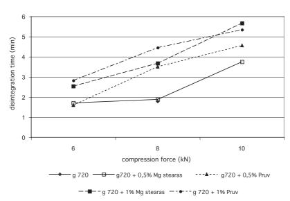
Fig. 3. Disintegration time in function of compression force: galen IQ 720 g 720 – galenIQ 720, g 721 – galenIQ 721, Mg stearas – magnesii stearas
