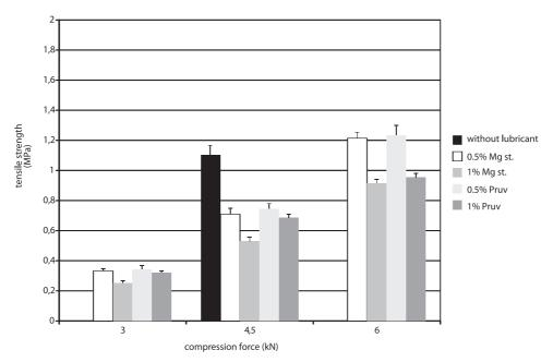
Fig. 3. Tensile strength of tablets in function of compression force: Sorbitab SD 500
