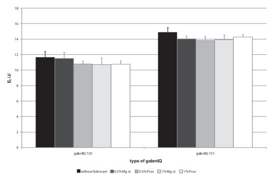
Fig. 2. Values of energy of friction at the compression force of 8 kN  $E_{\rm 1}$  – energy of friction, Mg st. – magnesium stearate
