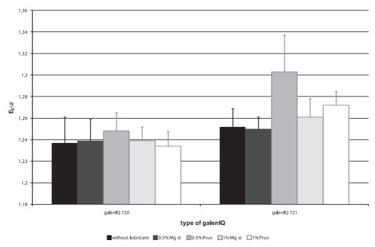
Fig. 4. Values of energy of decompression at the compression force of 8 kN  $E_z$  – energy of decompression, Mg st. – magnesium stearate
