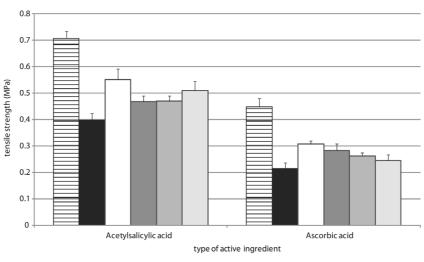
□ Prosolv SMCC 90 ■ Prosolv Easytab □ Prosolv SMCC 90+1%Explotab+0.5%Pruv □ Prosolv SMCC 90+15%Explotab+1.5%Explotab+0.5%Pruv □ Prosolv SMCC 90+1.5%Explotab+1.5%Explotab+0.5%Pruv □ Prosolv SMCC90+1.5%Explotab+1%Pruv
