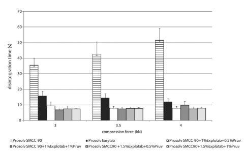
$Fig.\ 2.\ Disintegration\ time\ in\ function\ of\ compression\ force$
