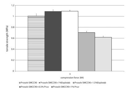
Fig. 3. Tensile strength of tablets at the compression force of 3 kN  $\,$
