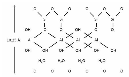
$Fig.\ 2.\ Schematic\ structure\ of\ hydrated\ halloysite\ (adapted\ according^{15)})$
