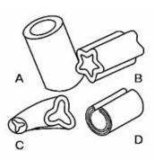
Fig. 3. Tubular carriers: A – cylindrical, B – star-like, C – triangular, D – multilayer horseshoe-like shape (adapted according<sup>32</sup>)
