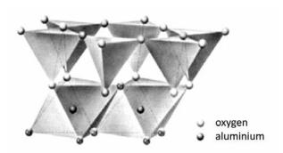
Fig. 1. Basic structural unit of halloysite (adapted according 32)
