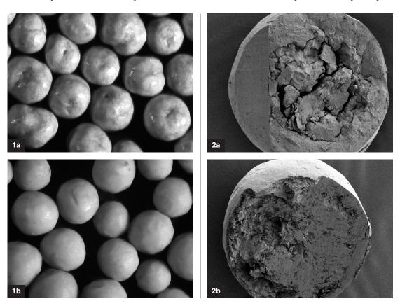
Fig. 4. The images of (a) drug-free and (b) drug-loaded halloysite pellets from (1) a light optical microscope (x 15) and (2) appropriate pellet cross-sections observed in a scanning electron microscope (x 80)
