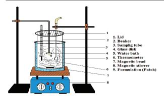
$Fig.\ 1.\ Modified\ dissolution\ apparatus\ used\ for\ in\ vitro\ release\ study$
