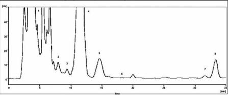
Fig. 1. HPLC chromatographic profile of dasylhydrazine derivatives of honey saccharides. Chromatographic conditions: see experimental part. 1 – dansylhydrazine, 2 – turanose, 3 – maltose, 4 – saccharose, glucose, 5 – fructose I, 6 – fructose II, 7, 8 – dansylhydrazine
