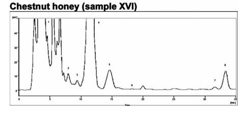
Fig. 1. HPLC chromatographic profile of dasylhydrazine derivatives of honey saccharides. Chromatographic conditions: see experimental part. 1 – dansylhydrazine, 2 – turanose, 3 – maltose, 4 – saccharose, glucose, 5 – fructose I, 6 – fructose II, 7, 8 – dansylhydrazine
