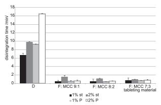
Fig. 4. Disintegration time of tablets at the compression force of 14 kN D – Disintequik<sup>TM</sup> MCC, F – Flowlac® 100, MCC – Microcel® MC-102, st – magnesium stearate, P – poloxamer 407
