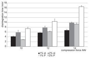
Fig. 3. Disintegration time of tablets in function of compression force – Disintequik  $^{\text{TM}}$  MCC with lubricants st – magnesium stearate, P – poloxamer 407
