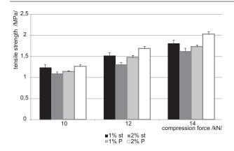
Fig. 1. Tensile strength of tablets in function of compression force – Disintequik  $^{\text{TM}}$  MCC with lubricants st – magnesium stearate, P – poloxamer 407
