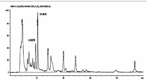
Graph 5. Determination of the positional specificity of lung cytosolic LOX. Reaction products were separated by RP-HPLC followed by SP-HPLC analysis of HETE by LOX from (AA)
