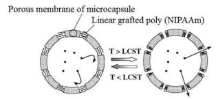
Fig. 8. The thermo-responsive release principle of the microcapsules with a porous membrane and the TR polymeric gates (modified from  $^{28)}$ )
