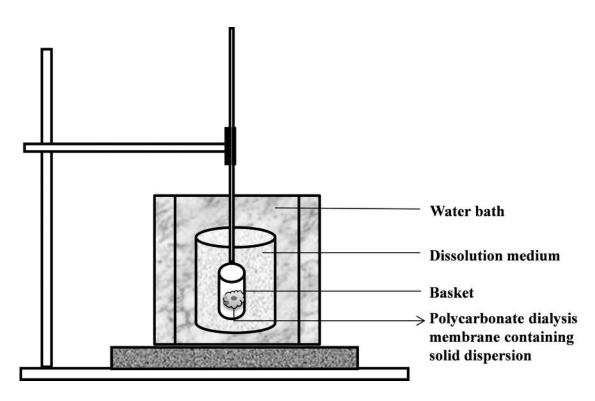
Fig. 1. Dissolution setup showing the placement of the polycarbonate dialysis membrane containing the solid dispersion in the basket
