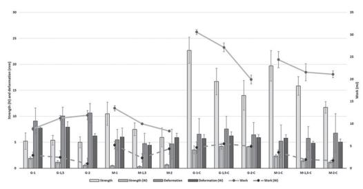
Fig. 5. Comparison of tested parameters observed through puncture testing (strength, work, deformation) in dry and wet states (W)
